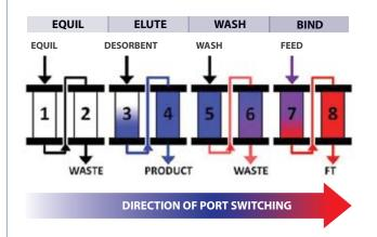
Step Mode uses multiple solvents and establishes independent zones to perform protocol steps analogous to conventional batch chromatography protocols but operated in a continuous cycle. At any given time, each zone performs one of the protocol steps resulting in simultaneous performance of multiple process steps. Programming flexibility enables users to create protocols employing up to eight Octave pumps in any combination to adjust flow rates, process times, and solvent compositions.
