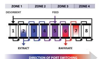
The solid phase is represented by individual columns connected in series, and the mobile phase by inlet streams of Feed and Desorbent and outlet streams of Raffinate and Extract. All four fluid streams are continuously fed into and withdrawn from the system. Streams are switched one column forward at each step of the cycle, timed to collect pure Extract (slower moving component) and Raffinate (faster moving component). The separation zone occupies 50-70% of the column material.
